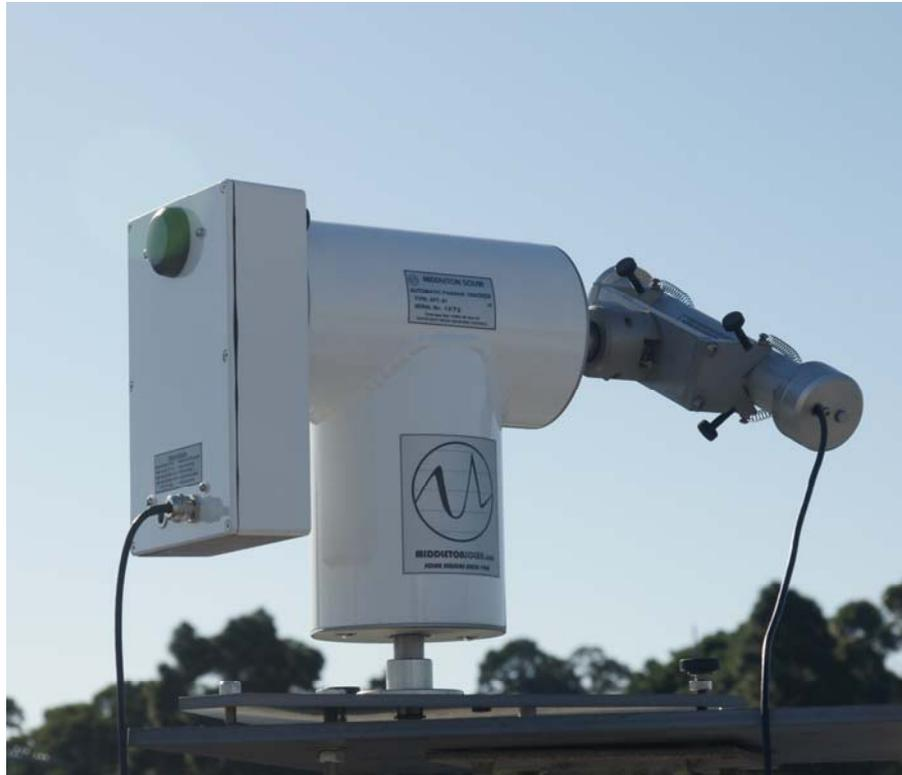
The Middleton Solar APT-01 is a 2-axis tracker to automatically point a solar pyrheliometer at the sun throughout the day. The APT-01 is a simple Passive Tracker and does without the closed-loop control Eye of the fully active AST-02/3 Tracker from which it is derived.
