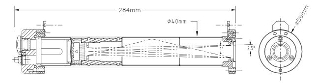
Exceeds the ISO9060 specifications for a First Class Pyrheliometer.
