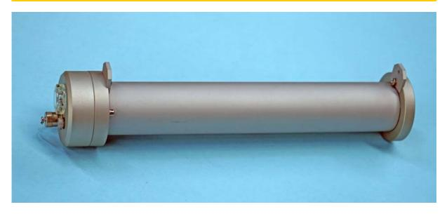
The Middleton Solar DN5 is an affordable precision pyrheliometer for measuring the solar direct radiation when aimed at the sun. It exceeds the international accepted specifications for a First Class pyrheliometer. The DN5 has a passive microvolt output, and the DN5-E version has an in-built amplifier to give a millivolt output for easy signal measurement.
