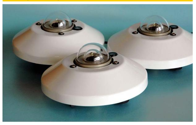
The Middleton EQ08-S exceeds all international accepted specifications for a high quality pyranometer. The EQ08-S incorporates a unique thermoelectric sensor that has exceptionally low directional error without compromise to signal strength or response time. The EQ08-SE version has an in-built amplifier to give a millivolt output for easy signal measurement.
