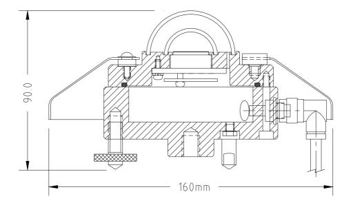
Exceeds every ISO 9060 parameter for a Secondary Standard Pyranometer.
