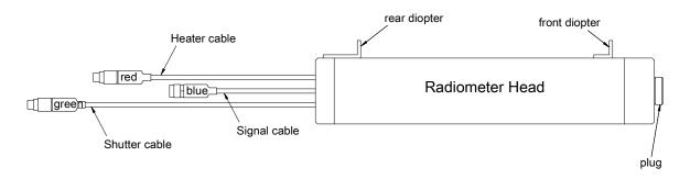
The Radiometer Head has three short cable tails with colour-coded connectors. The three Interface Leads, each 6m long, should be coupled to the appropriate coloured tail connector; allow sufficient slack so the Interface Cables do not become taut during operation of the Solar Tracker.
