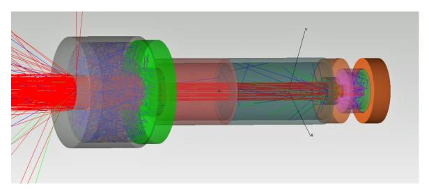
The above image is a simplified 300-ray simulation of a model of the complete ACR-01 Radiometer Head; it illustrates the ray trajectories in the whole instrument.
