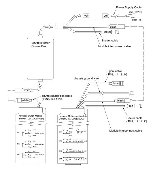
Fit the supplied Signal cable (P/No 141.1114) and Heater cable (P/No 141.1113) to the Keysight 34901A (or DAQM901A) Multiplexer Module. Fit the Shutter/Heater Box cable (P/No. 141.1110) to the Keysight 34903A (or DAQM903A) Switch Module.
