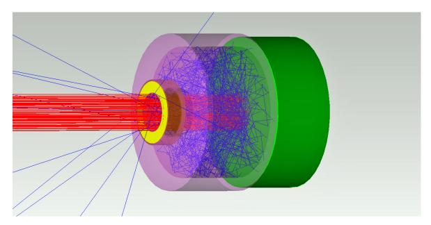
The above image is a simplified 150-ray computer simulation of a model of the detector cavity; it illustrates the ray trajectories in the cavity.
