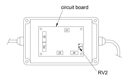
The heater power is set using potentiometer RV2. The recommended nominal heater power is 1,000 W.m-2. The available adjustment range is approximately 950 to 1,100 W.m-2.
