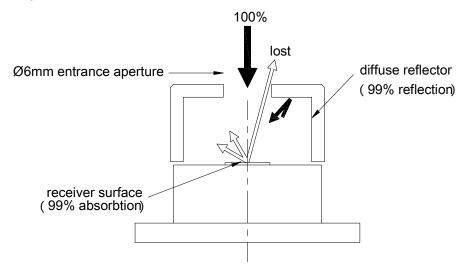
Of the solar radiation entering the front detector cavity, approximately 99% is absorbed by the black Carbon Nanotube receiver surface, and 1% is back-scattered<sup>10</sup>. Some of the back-scattered radiation is lost through the entrance aperture, and most of the remainder is returned to the receiver surface by the reflector.
