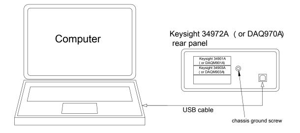
Insert the two Modules into the Keysight Data Acquisition Unit. The Multiplexer Module (\*\*901A) into the top slot, and the Switch Module (\*\*903A) into the middle slot.
