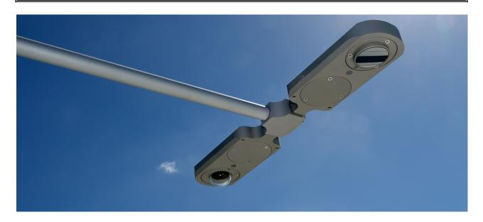
The Middleton Solar **NSK4** is a 4-component **Net Radiometer** to measure solar & thermal radiation downward and upward, through a horizontal plane. It has four thermoelectric sensors, two are shielded by glass domes and two by silicon windows. The glass domes are transparent to shortwave (SW) solar radiation and the silicon windows are transparent to longwave (LW) radiation emitted by the atmosphere or the Earth surface.
