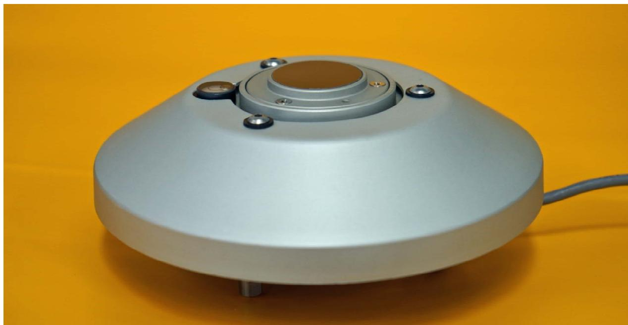
The Middleton Solar PG01 Pyrgeometer is for measuring long wave radiation emitted by the atmosphere (downwelling) or the Earth surface (upwelling). It uses a passive thermoelectric sensor shielded by a flat silicon window. The window is coated to exclude radiation below 4.5  $\mu\text{m}$ . The PG01 is sealed and fully weatherproof.
