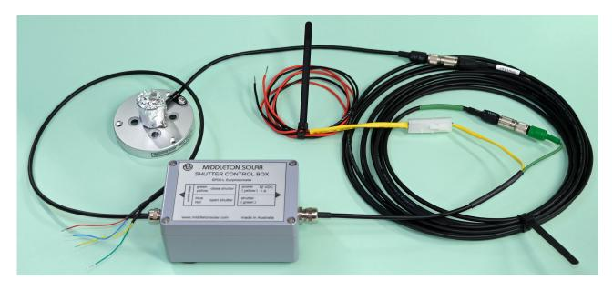
Attach the supplied 'yellow' 12V power cable to the Control Box.
