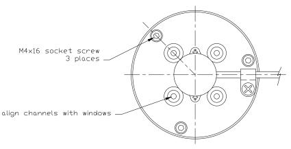
Fit the Shutter using three supplied M4x16 socket screws. Align the four Sunphotometer channels with the windows.
