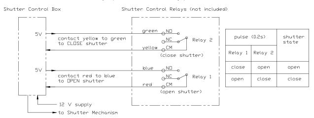
Connect the 'yellow' power cable to a 12 VDC supply (not included); red wire to +ve.
